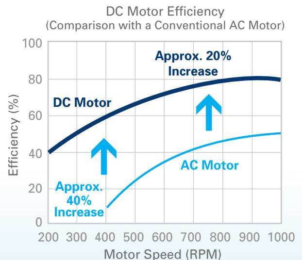
Note: Data is based on studies conducted under controlled conditions at a Daikin laboratory.
